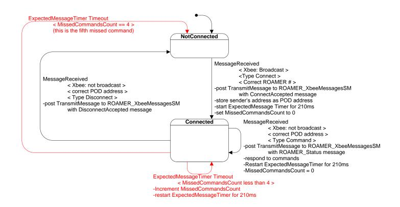
The receive interrupt should post MessageReceived to the ROAMER\_CommunicationSM when it receives an incoming message API (0x81). The ROAMER will ignore anything except Connect requests when not connected. It will then respond to the first POD to send a connection request with its ROAMER number. Once connected, it will ignore any connection requests and any messages not from its POD.
