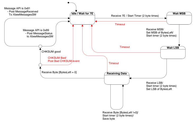
This is a simple state machine to process incoming messages. It should work with the async receive interrupt, putting bytes in the correct location as they come in. Once the message is complete and the checksum is checked, the state machine should route the message to either the XbeeMessagesSM or the CommunicationSM. Red transitions represent error is receiving the message, and should be handled for debugging.
